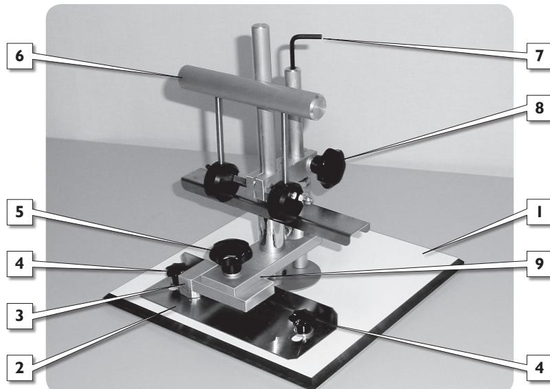
The stamping height can be adjusted by loosening the adjustment knob (8) and moving this knob upwards or downwards.
